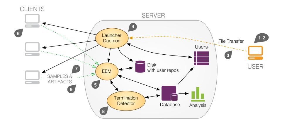
8) Termination Detector evaluates body of samples; when termination condition reached, tells EEM to send shutdown message to SCs.
