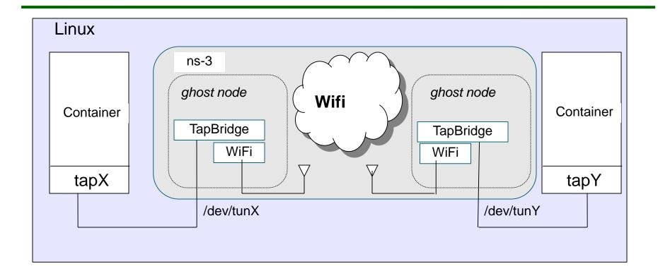
Tap device pushed into namespaces; no bridging needed
