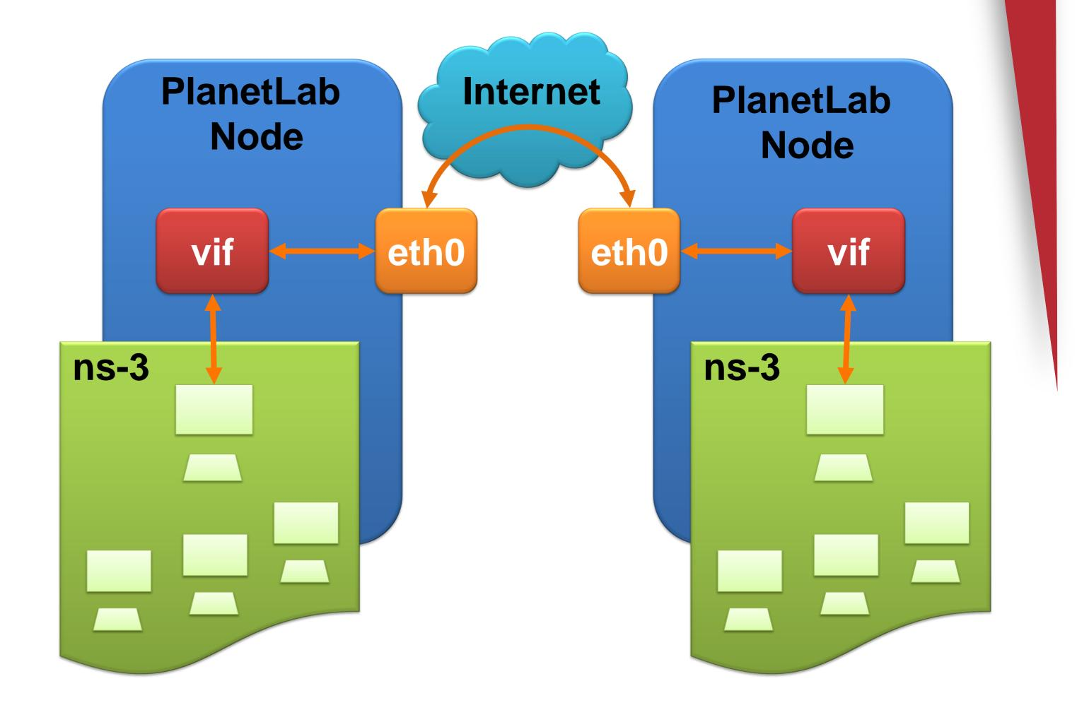
**management tool** that enables conducting heterogeneous experiments where PlanetLab nodes and Emulated nodes can be seamlessly integrated with ns-3 simulations.
