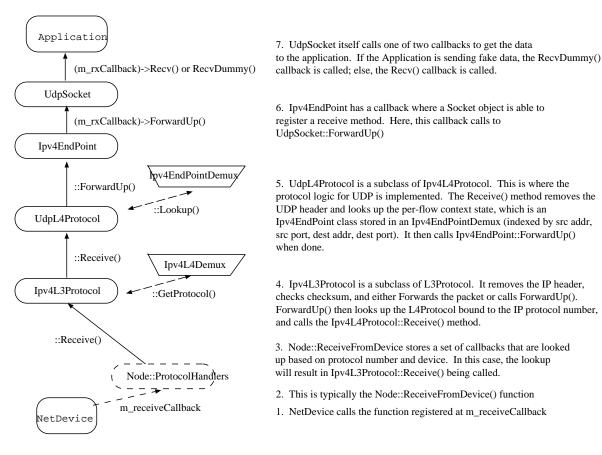
Figure 5.2: Steps in the receive packet processing chain (Ipv4/UDP example).
