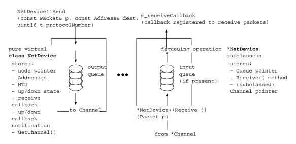
Figure 3.2: Overview of boundary between Network Device and upper layer (typically layer-3).
