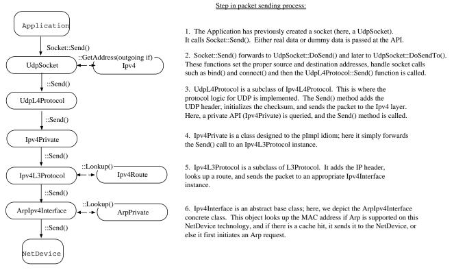
Figure 5.1: Steps in the send packet processing chain (Ipv4/UDP example).
