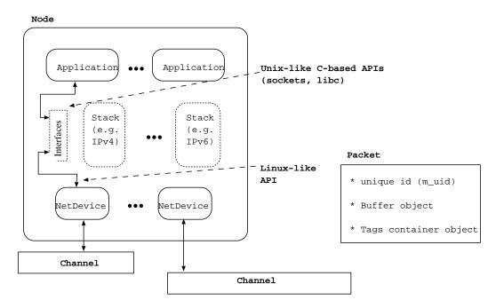
Figure 3.1: High-level node architecture.
