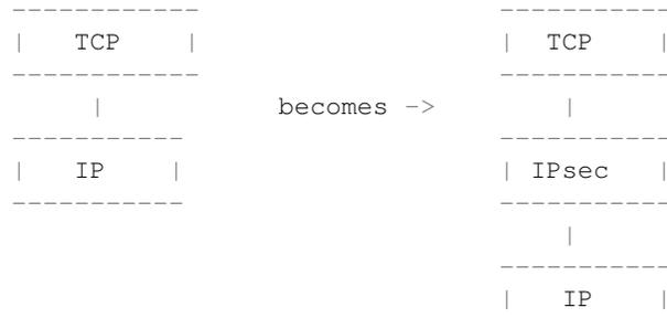
If the simulator has made assumptions, and hard coded into the code, that IP always talks to a transport protocol above, the user may be forced to hack the system to get the desired interconnections. This is clearly not an optimal way to design a generic simulator.
