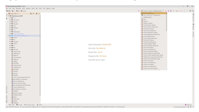
If you have selected and executable target, you can click either the play button to execute the program; the bug to debug the program; the play button with a chip, to run Valgrind and analyze memory usage, leaks and so on.
