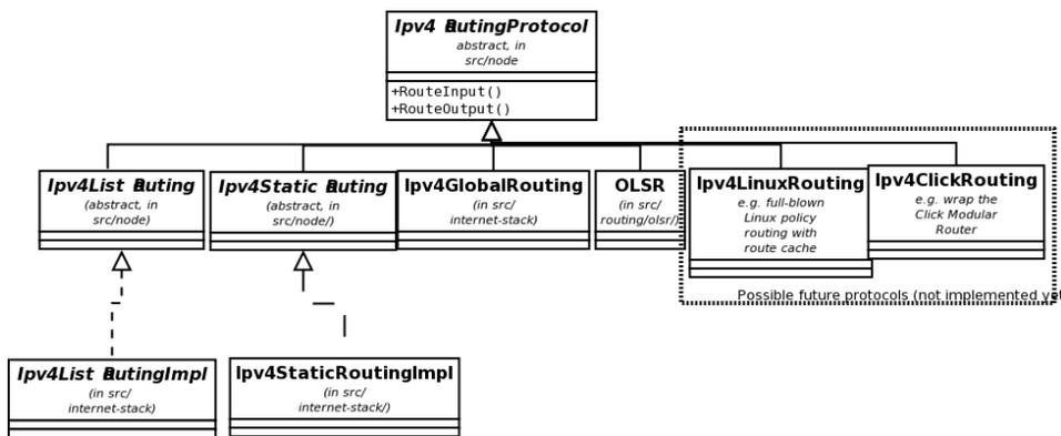
Figure 29.2: `Ipv4Routing` specialization
