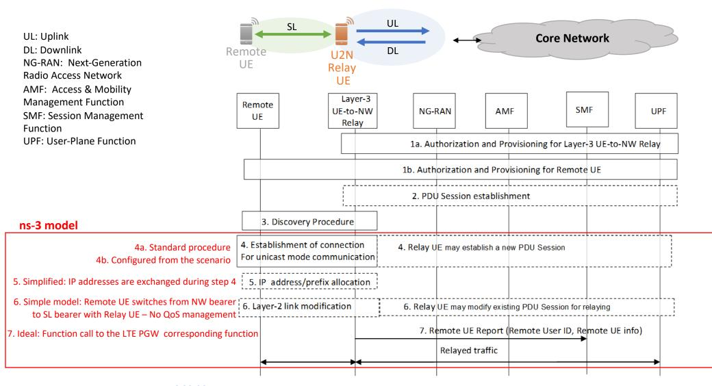
TS 23.304 Figure 6.5.1.1-1: 5G ProSe Communication via 5G ProSe Layer-3 UE-to-Network Relay without N3IWF
