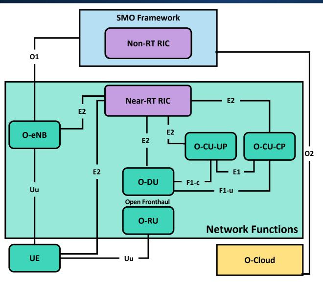
Serves as the logical link between E2 nodes and the Near-RT RIC (E2 node is any RAN component with an E2 interface between itself and the Near-RT RIC)
