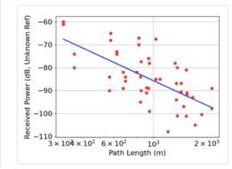
The figure shows the received power (red dots) vs. path length for 56 links between pairs of CBRS rooftop nodes. The dB received power is not calibrated, so is listed as referred to an unknown reference. The path loss exponent model for the measurements (blue line) has a path loss exponent of 3.6 and standard deviation of 8.5 dB.
